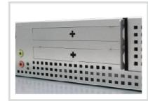
1 x PCle x1 slot and 1 x PCle x16 slot
