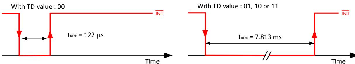
Figure 6: Auto reset time  $t_{RTN1}$  profiles according to TD values
