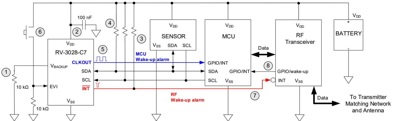
Figure 4: Example of Wireless Sensor Node (WSN) with wake-up managed by RV-3028-C7 RTC Module
