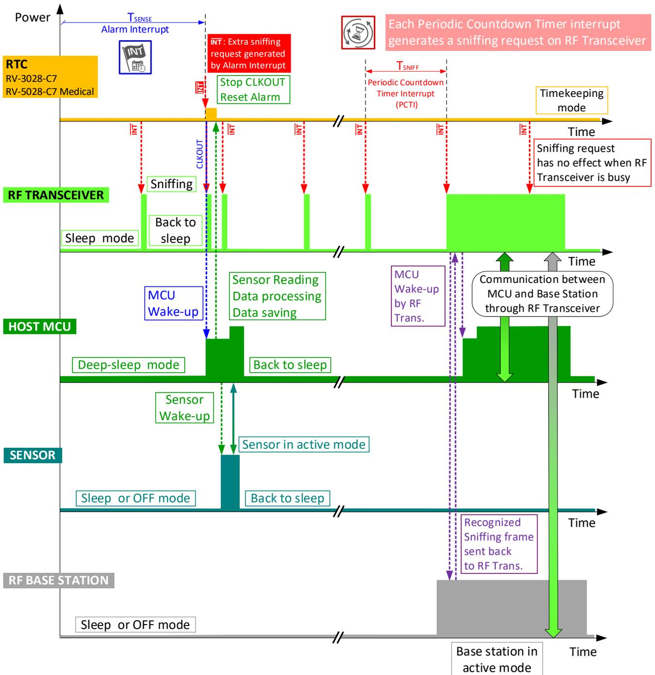
Figure 8: WSN activity chart when using an RTC
