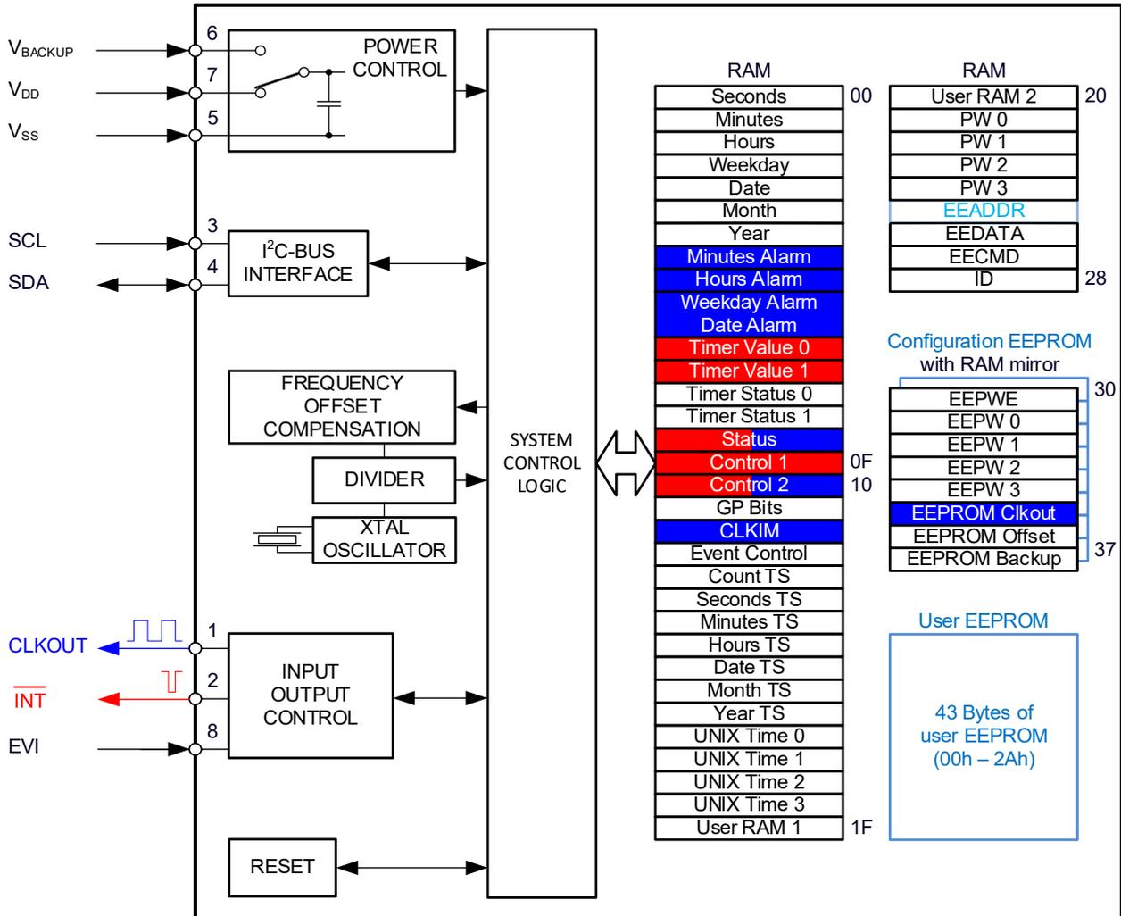
Figure 3: RV-3028-C7 Block Diagram
