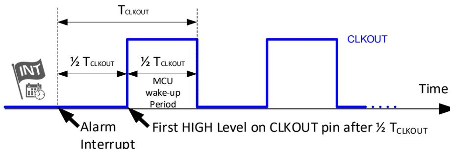
Figure 5: CLKOUT profile once Alarm Interrupt occurs
