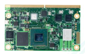
The i.MX 95 SoC based SMARC System On Module is designed as per SMARC specification v2.1.1. It integrates NXP's i.MX 95 offerings, 6x Arm Cortex A55 @ 1.8GHz, 1x Arm Cortex-M33, 1x Arm Cortex-M7, NPU with up to 2.0 TOP/s and IEEE 802.11 a/b/g/n/ac/ax Wi Fi + Bluetooth 5.3 module.
