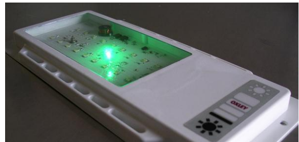
Integrated green LED for blackout IR secure operations
