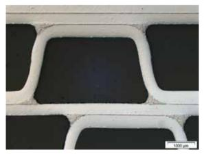
A micrograph of the cross section of a stainless steel EGR cooler brazed with VITROBRAZE VZ2170
