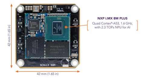
The flagship SoM board of the SCAiLX platform is built on an NXP i.MX 8M Plus processor with an integrated Neural Processing Unit (NPU). The i.MX 8M Plus processors are designed to excel in Al machine learning and vision applications.
