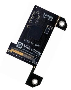
Broaden the functionality of the SCAiLX platform by integrating Videology Zoom Block cameras using the SCAILX-LVDS-2-MIPI board.
