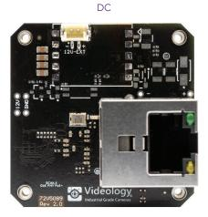
Enhance your SCAiLX Edge AI modular platform with our connectivity and power boards. Both the Power over Ethernet (PoE) and DC powered Ethernet boards measure 42x42 mm, perfectly matching the dimensions of other SCAiLX modular platform boards. These Ethernet interface boards facilitate fast and easy camera powering and connectivity.
