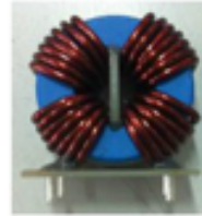
2x14.2mH/16Arms Isolation 1500Vac 33x31.5x20mm (nanocrystalline)
