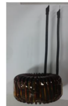
90x55mm single 7kW PFC choke 235µH/32Arms/100kHz (sendust)
